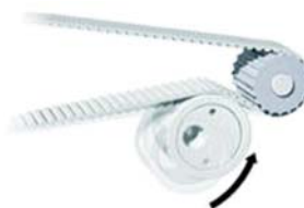
Mounting instruction: counter-clockwise tensioning!
